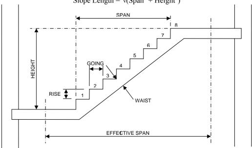
When the flight is built monolithically into members spanning at right angles to its span, the effective span is given by:
